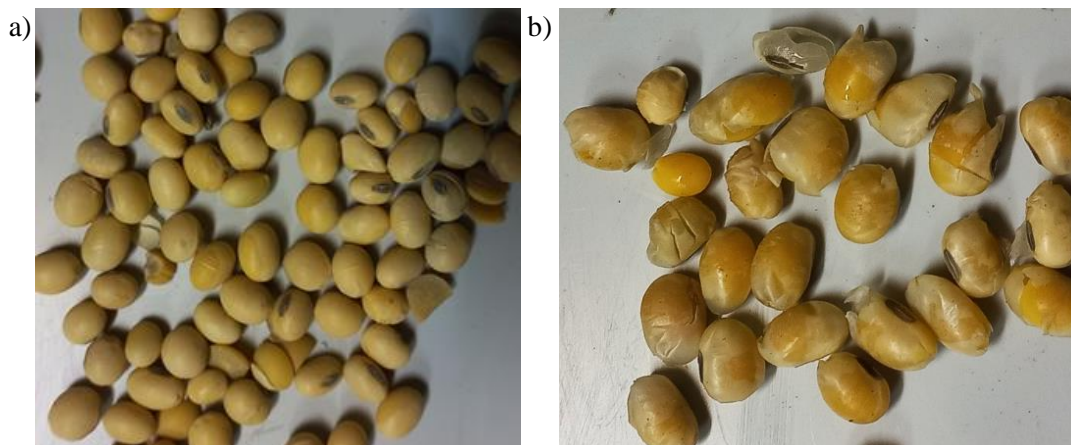
Fig. 4. Appearance of soybean seeds after drying at vacuum value more than critical (a) and less than critical (b) at temperature 30 °C
